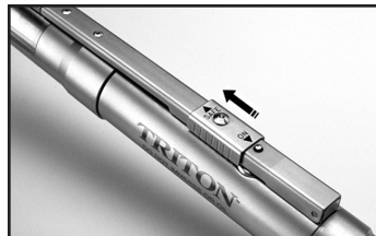
“SAFE”: Lift Finger Control and push “Safety Slide” away from “ON” position.
