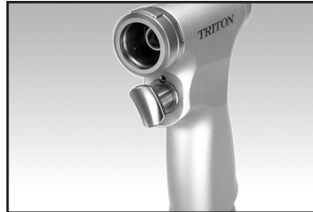
“SAFE”: Turn Trigger Control to either side.
