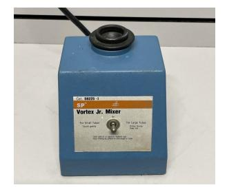
Vortex mixers are commonly used in laboratories to mix small liquid volumes for cell disruption or homogenization. The analog or digital vortex mixers precisely control the operational speed and time to achieve reproducible results.
